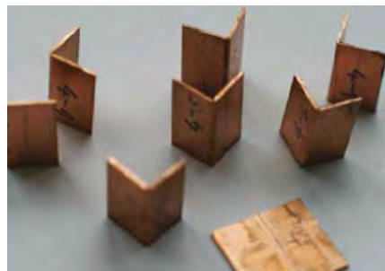
Longitudinal and cross-ways bending tests of the weld seam, radius 1.00 mm, 90° angle
