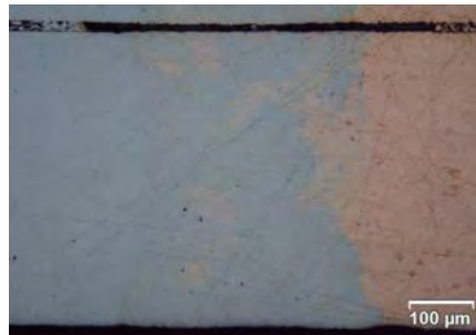
Polished sample of weld seam of copper-steel-combination
